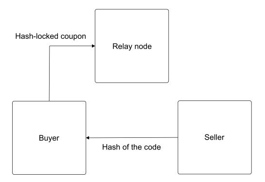
The buyer-to-relay and relay-to-seller routes are secured by CLTV payment channels. Once the seller unlocks the funds, the code is set to be automatically disclosed by the contract:
